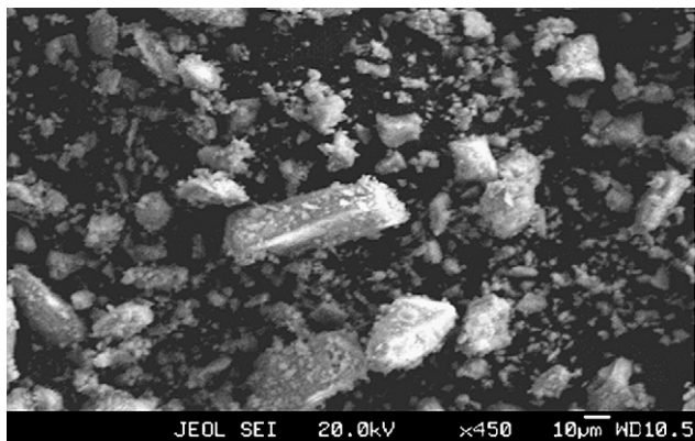
Fig. 6. Scanning electron micrograph of 15 wt.% ZPTA sample.
